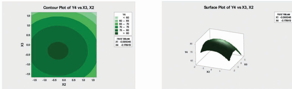
Plot Contour and Surface Response at Conditions X_1 and X_3 at the Stationary point
