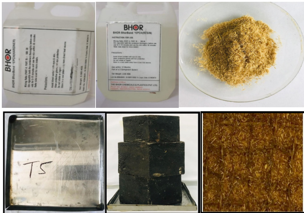
Fig. 1(a) Epoxy Resin (b) Hardener (c) Rice straw fiber (d) mold design, (e) mold with a RS reinforced bio-composite with a pressure system (f) specimens of bio-composites reinforced with surface modified RS
