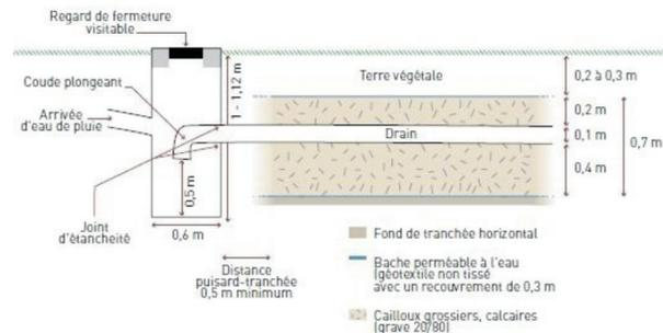
**Fig. 2.** Example of a drainage trench.
