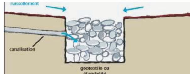
**Fig. 3.** Structural sections of drainage structure.
