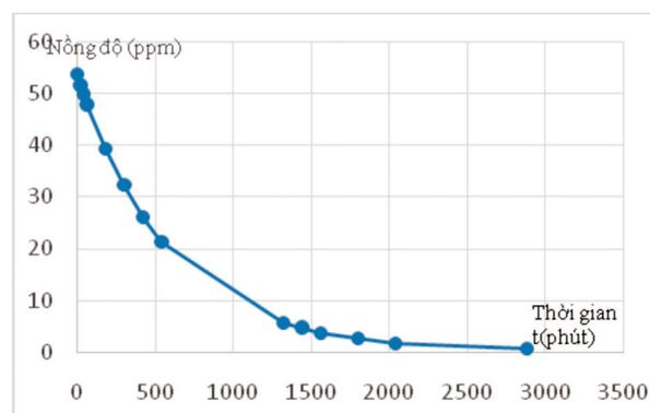
Fig. 4. Acenaphthylenetreatment by doped TiO<sub>2</sub>
