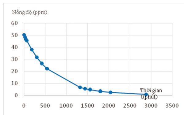
**Fig. 5.** Acenaphthenetreatment by doped  $\text{TiO}_2$
