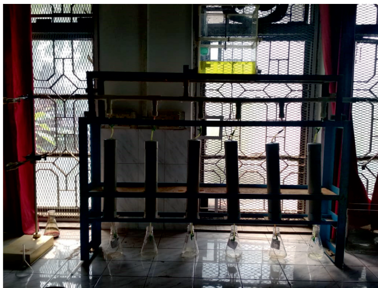
Fig. 1. Lab Scale Chromium adsorption column
