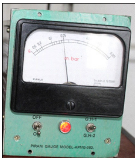
Fig. 6. Pirani gauge for lower vacuum measurement
