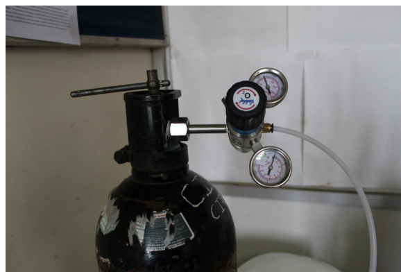
Fig. 7. Nitrogen gas cylinder and its regulator system
