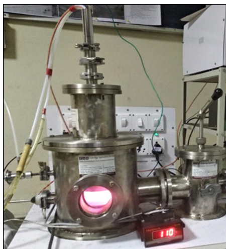
Fig. 8. K type thermocouple mounted in the chamber
