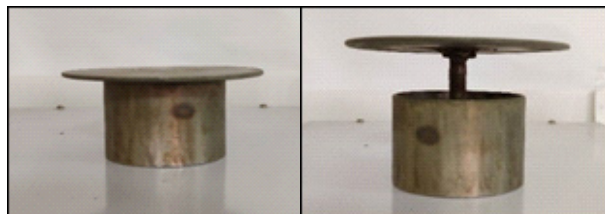
Fig. 3. Adjustable sample holder present in the plasma chamber
