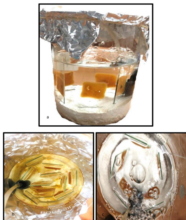
Fig. 2(a-c). Set up of immobilized system for biooxidation; b- Placement of the slides inside the beaker; c-external aeration as seen from the top
