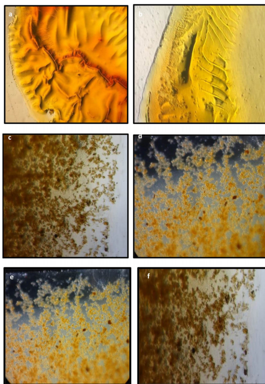
Fig. 3(a-f). a,b-Film of Gold formed after dissolving in aquaregia indicating the formation of Gold; (c-f)- Gold formed at all the edges of the slide
