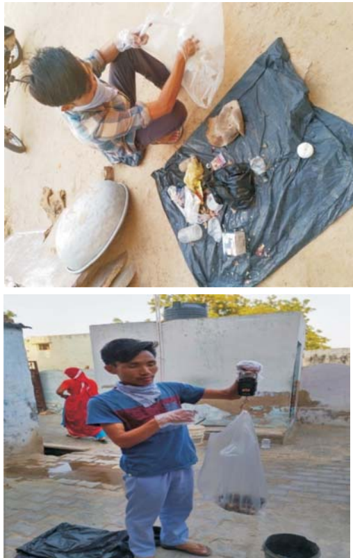
Fig. 1 & 2. Picture depicting manually hand sorting and weighing of solid waste
