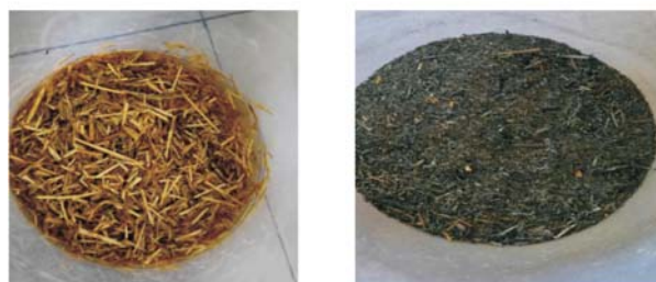
C. Developed adsorbent after chemical and thermal treatment
