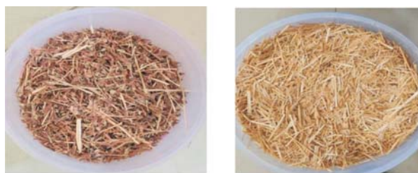
A. Procurement and drying of pigeon pea husk and wheat husk
