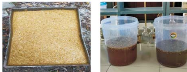
B. Washing and soaking of agricultural material PPH and WH
