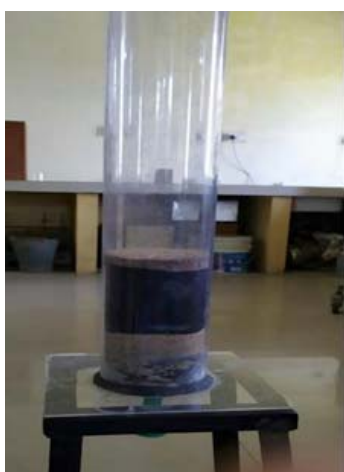
Fig. 2. Filter unit containing adsorbent as filter media
