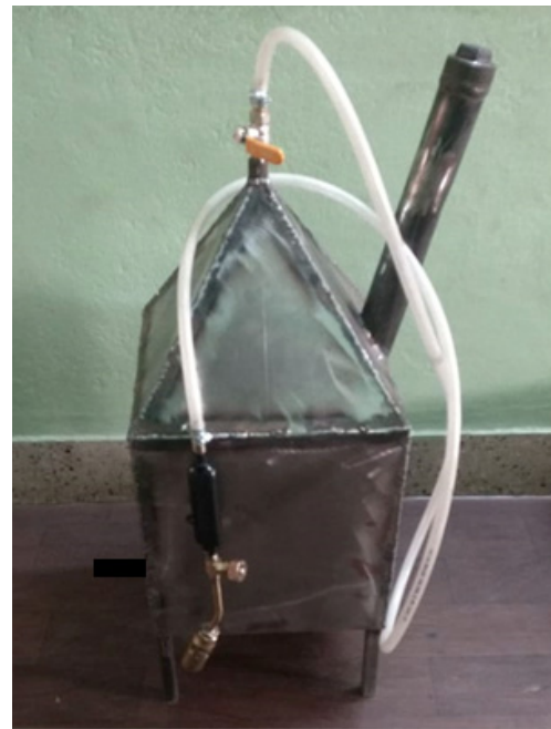
Fig. 2. Fabricated biogas digester for fermentation process
