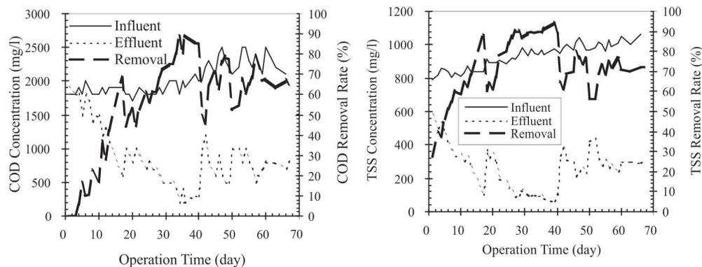
Fig. 2. Performance of the AFBR in removing COD and TSS from wastewater
