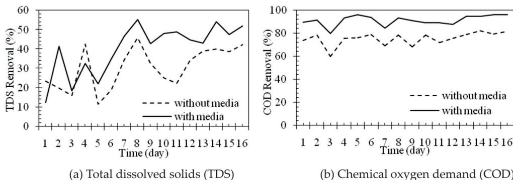
Fig. 2. Comparative removal efficiency of TDS and COD in the reactor.
