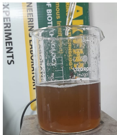
Fig. 4. Synthesis of ZnO nanoparticle from zinc nitrate dihydrate using O. tenuiflorum extract
