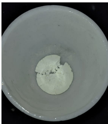
Fig. 7. Calcinated ZnO nano particle powder.
