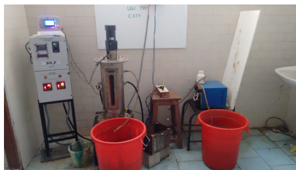
Fig. 2. Experimental set up of Continuous Stirred Tank Reactor
