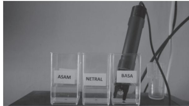
Fig. 8. Verification process between pH sensor and Probe Sensor using Buffer pH Solution
