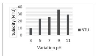
**Fig. 4.** Final turbidity value (NTU) for the coagulant of papaya seed powder at pH variations
