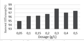
Fig. 1. Removal efficiency of turbidity with papaya seed coagulant
