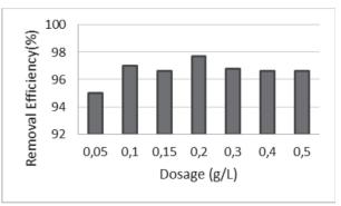
Fig. 2. Removal efficiency of turbidity with powder coagulant of papaya seeds
