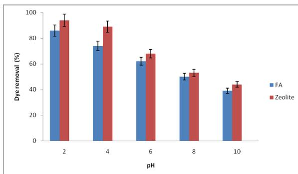
Fig. 3. Adsorption of Acid violet 19 dye by coal fly ash and zeolite at different pH.
