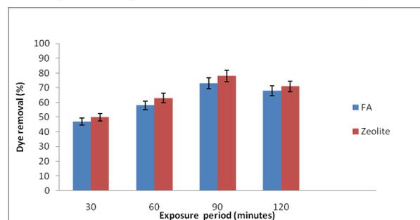
**Fig. 1.** Adsorption of Acid violet 19 dye by coal fly ash and zeolite at different exposure period.
