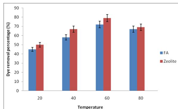
Fig. 4. Adsorption of Acid violet 19 dye by coal fly ash and zeolite at different temperature.
