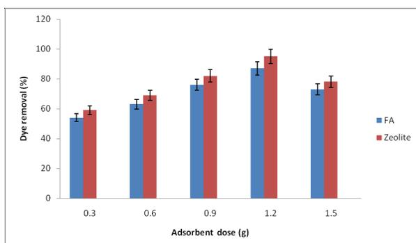
Fig. 2. Adsorption of Acid violet 19 dye by different adsorbent dose.
