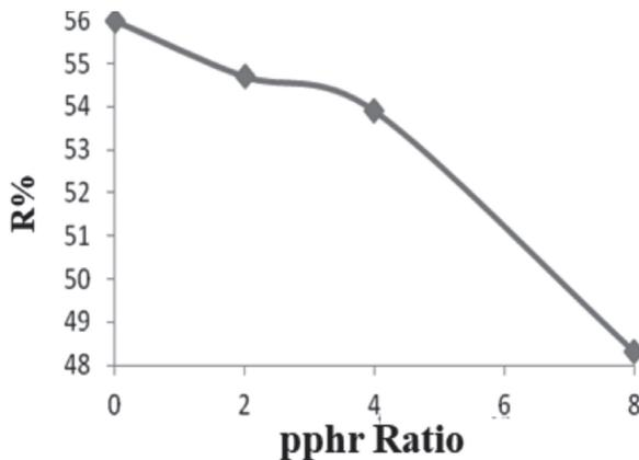
Fig. 7. Effect of increasing  $\text{MgFe}_2\text{O}_4$  in the rubber composite on the wave reflection ratio.
