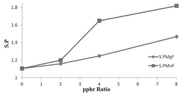
Fig. 3. Specific gravity (S.P) variation with pphr ratio in the composite rubber.
