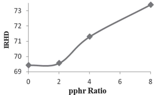
Fig. 5. Effect of increasing  $MgFe_2O_4$  in the rubber composite on the hardness.
