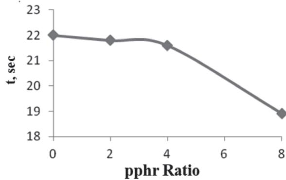
Fig. 8. Effect of increasing  $\text{MgFe}_2\text{O}_4$  in the rubber composite on the damping time.
