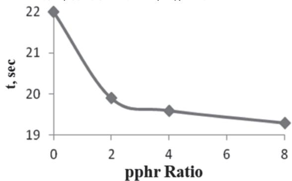
Fig. 9. Effect of increasing  $\text{MnFe}_2\text{O}_4$  in the rubber composite on the damping time.
