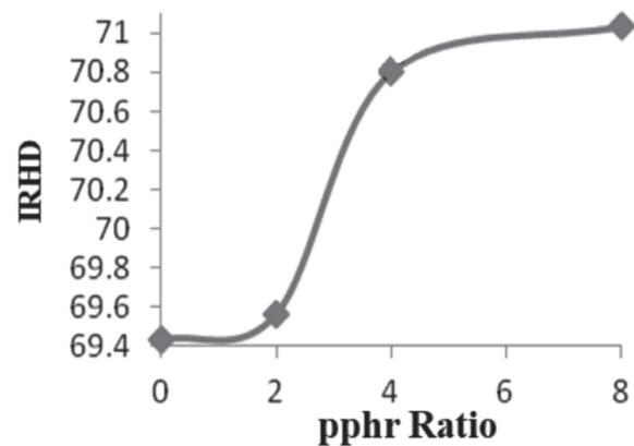
Fig. 4. Effect of increasing  $MnFe_2O_4$  in the rubber composite on the hardness.
