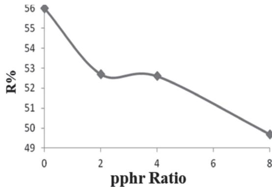
Fig. 6. Effect of increasing  $\text{MnFe}_2\text{O}_4$  in the rubber composite on the wave reflection ratio.
