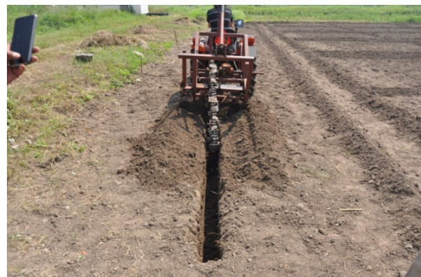
Fig. 3. Field operation of prototype trencher
