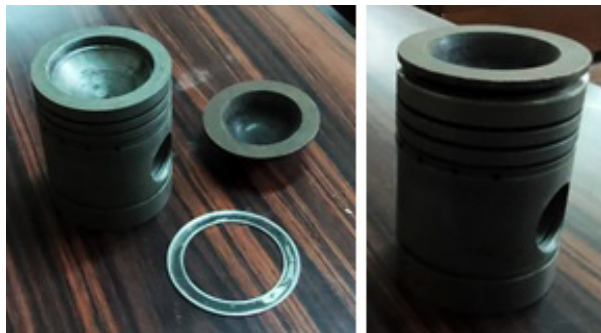
Fig. 2. Photographic view of air gap insulated piston
