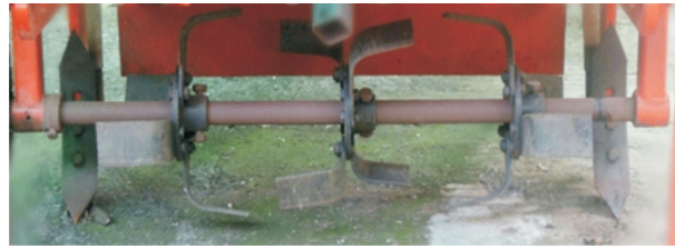
Fig. 4. Developed rotor blade shaft assembly
