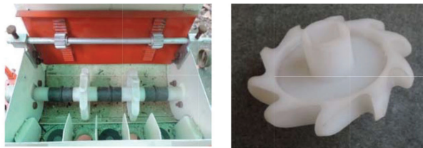
Fig. 6. Detailed view of fertilizer metering mechanism
