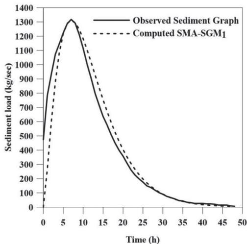
Fig. 3. Observed vs. Computed Sediment Graph of Validation Event (21-22/08/1983)
