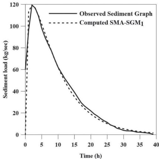
Fig. 2. Observed vs. Computed Sediment Graph of Calibration Event (24-26/07/1982)
