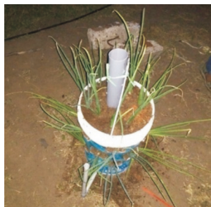
Fig. 2. Fabricated and onionseedling transplanted low cost self-irrigated container
