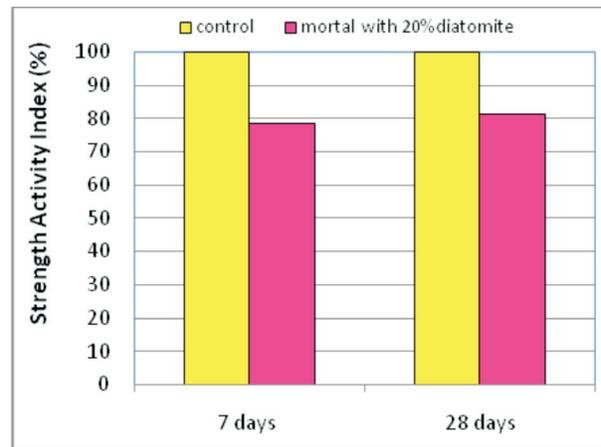
Fig. 4. Strength activity index of diatomite
