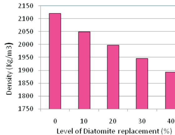
Fig. 8. Density development of mortars containing various amount of diatomite
