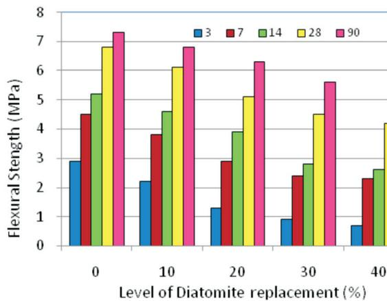
Fig. 6. Flexural strength development of mortars containing various amount of diatomite
