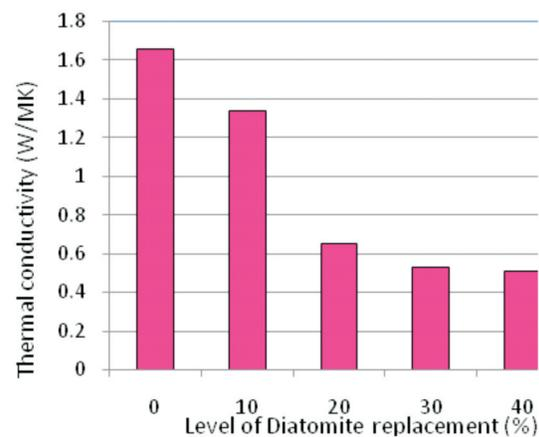
Fig. 9. Thermal conductivity of mortars with various level of diatomite replacement
