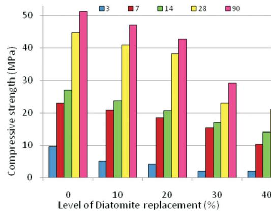
Fig. 5. Compressive strength development of mortars containing various amount of diatomite
