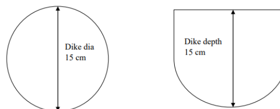
Fig. 4. Dimensions of dikes formed in the crop rows
