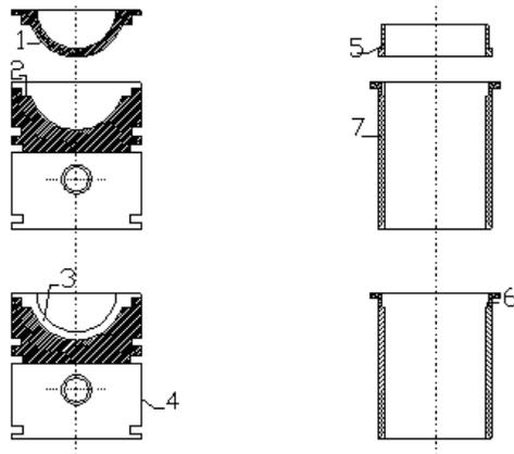
**Fig. 1.** Assembly details of air gap insulated piston and air gap insulated liner
