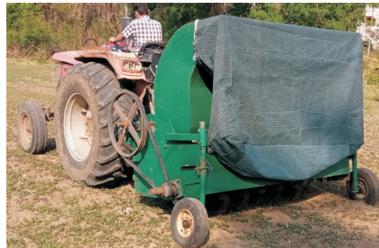
Fig. 4. Cotton stalk harvesting machine with collecting unit
