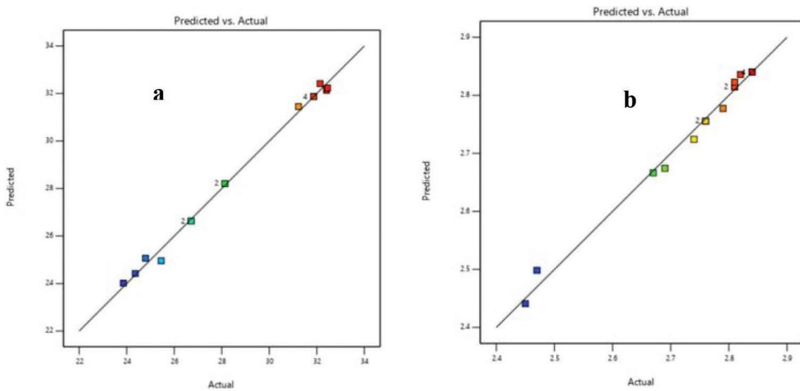
Figure 4. Relationship between actual and predicted values of (a) Carbon content (b) Nitrogen content
