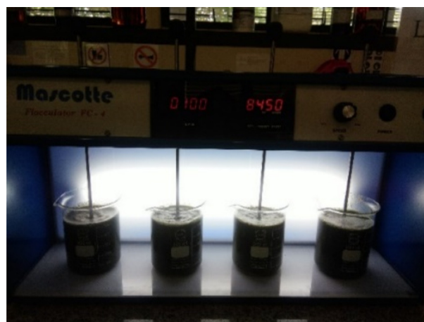
Fig. 1. Process of Laying Wastewater Samples and Adsorbents for 90 minutes
