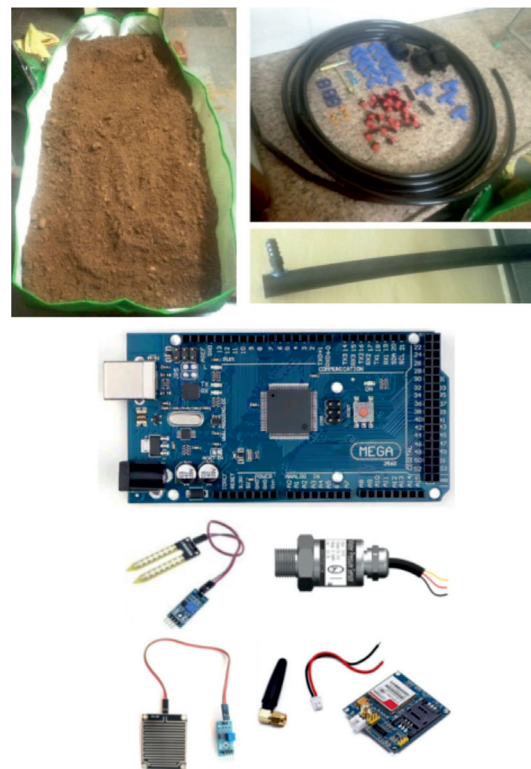
Fig. 1. Experimental Setup HDPE Grow Bag (6 X 3 feet), Drip Irrigation Kit, and IoT Sensors (Initial Stage)
