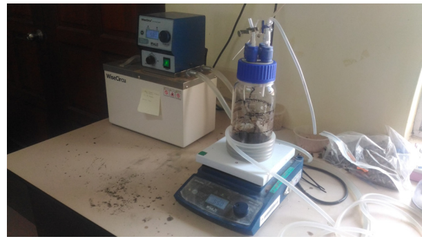
Fig. 1. Experimental setup of anaerobic digestion of AWW.
