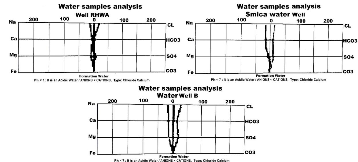
Fig. 4. Stiff diagram water samples analysis.
