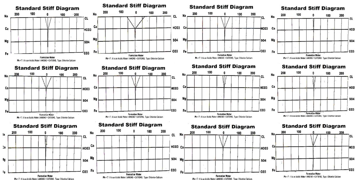
Fig. 6. Stiff diagram of water analyses associated with gas production.
