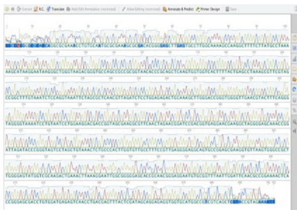
Fig. 5c. Sequence chromatogram of the PCR product by Geneious Prime Software; green color represents thymine (T); yellow, guanine (G); red, adenine (A); blue, cytosine (C). Highlighted parts mean that the chromatogram could not separate clearly the signal from noise and the software had to remove the noise.
