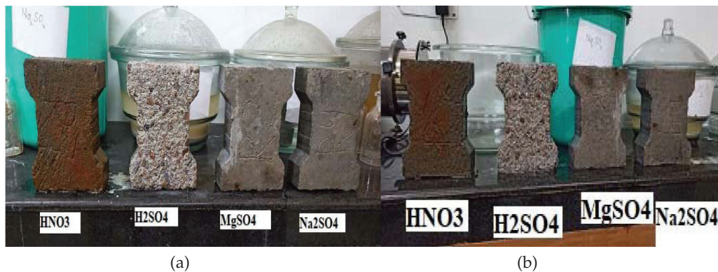
Fig. 4. Control Mix concrete (MR-0) Paver Blocks after (a) 0 days; (b) 30 days; (c) 60 days; (d) 90 days
