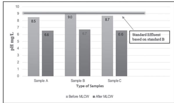
**Fig. 2.** Different of pH between before MLCW and after MLCW
