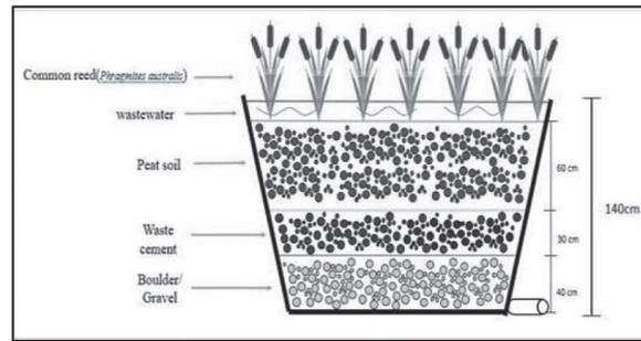
**Fig. 1.** Filling materials in multi-layer constructed wetland
