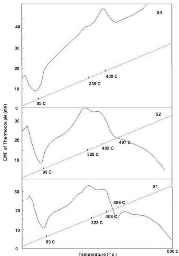
Fig. 2. DTA curve for soil samples
