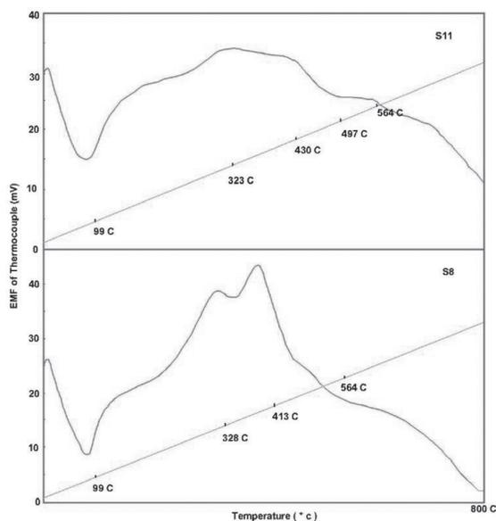
Fig. 1. DTA curve for soil samples
