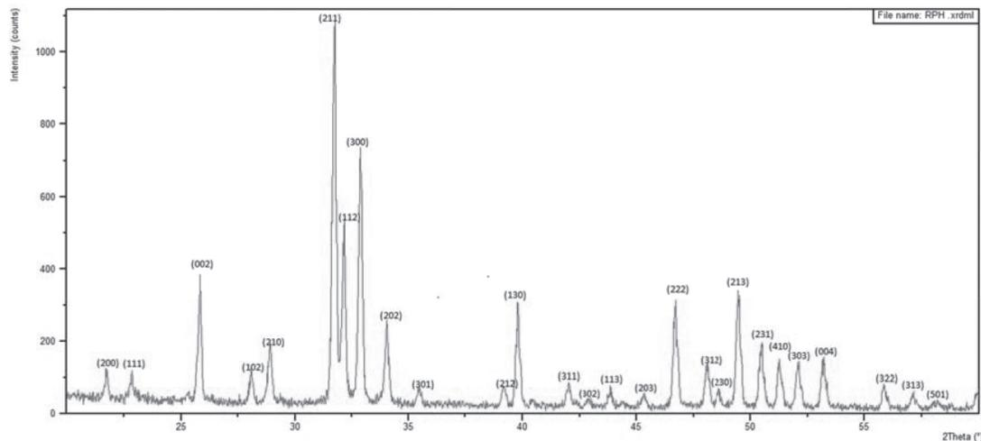
Fig. 3. XRD testing data of BHA sample
