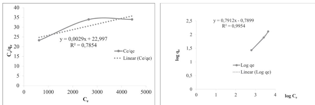
Fig. 4. Langmuir (right) and Freundlich (left) for activated carbon immobilized alginate of adsorption isotherms
