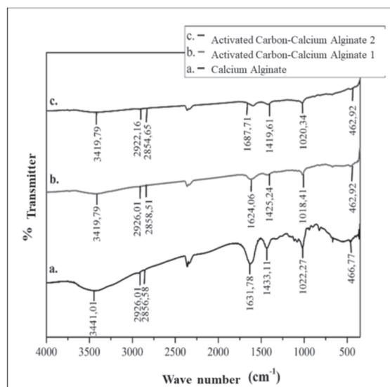
Fig. 1. FTIR Spectra (a) adsorbent of calcium alginate (b) adsorbent of activated carbon-calcium alginate 1 (before decolorization) and (c) adsorbent of activated carbon-calcium alginate 2 (after decolorization)
