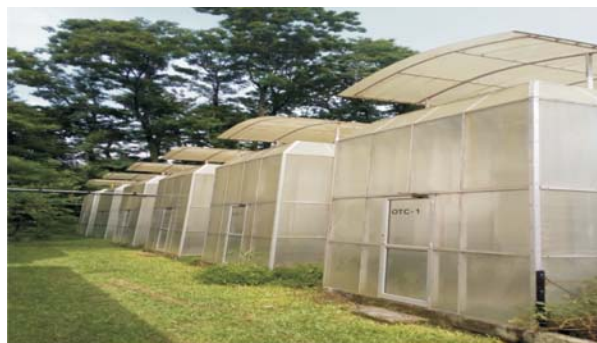
Fig. 3. Open top chamber facility of different concentration of CO 2 in Forest Research Center, Dehradun
