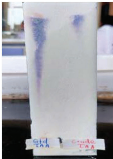
Fig. 2. TLC analysis of IAA production by Isolate IS-2
