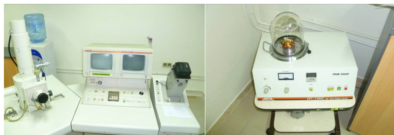
Fig. 8. The scanning electron microscope with the sputtering device used
