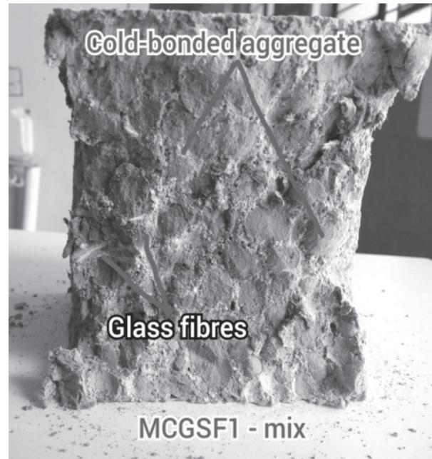
Fig 12. MCGSF1 – Tested Specimen
