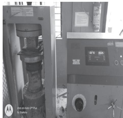
**Fig 5.** Universal Testing Machine
