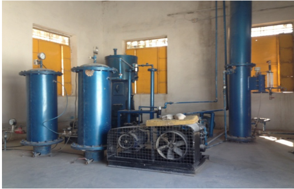
Fig. 2. View of Biogas upgrading unit with water scrubbing column and compressor unit at experimental site
