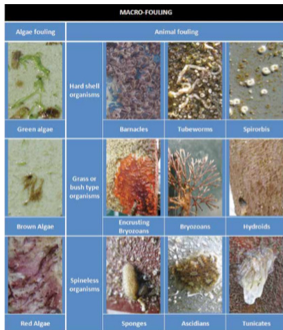
Fig. 4. Types of Biofouling; (A) algae fouling: green algae, brown algae and red algae; (B) animal fouling: barnacle, tubeworm, spirobrans, encrusting bryozoans, bryozoans, hydroids, sponges, ascidians, and tunicates (Bressy and Lejars, 2014).
