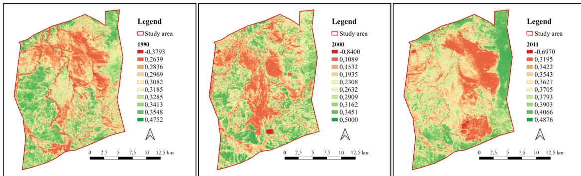
Fig. 7. NDVI on the vegetation distribution in 1990, 2000 and 2011 calculated from Landsat-5 TM
