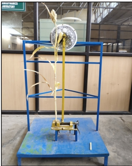
Plate 1. Determination of cutting energy requirement of crop by pendulum impact tester
