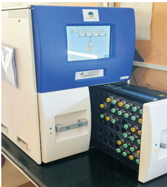
Fig. 1. Bactec instrument (Automated Blood Culture System utilizes fluorescent technology in detecting the growth of organisms in the blood culture bottles)
