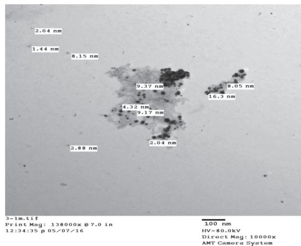
Fig. 2. TEM image of *G. thermodenitrificans* AZ1 produced extracellularly.
