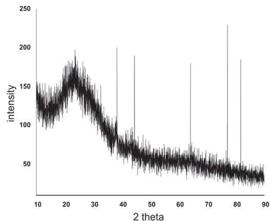
Fig. 4. XRD pattern of AgNPs synthesized by culture supernatant of *G. thermodentrificans* AZ1
