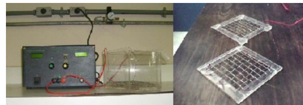
Fig. 2. Experimental Electro flotation unit and stainless-steel mesh electrode Source: (Motaa et al. , 2015)
